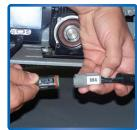
Weather proof, labeled electrical quick connectors are used for safety and offer understandable & easy machine servicing.
