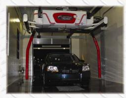
To keep Vector running smoothly, its carriage head moves on overhead travel rails that keep its motors and gears up away from dirt and grime. The swivel-free design, all-electric drive and greased-for-life bearings reduce complexity and maintenance costs. Which all underscores Vector's design premise: "If maintenance is easy, it will get done!"
